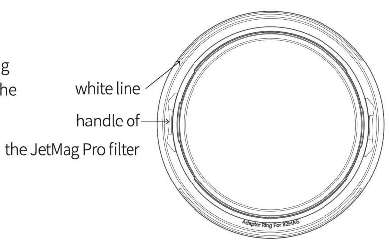
4. Rotate the holder until the JetMag Pro filter handle aligns with the white line. This will lock the main adapter in place.
