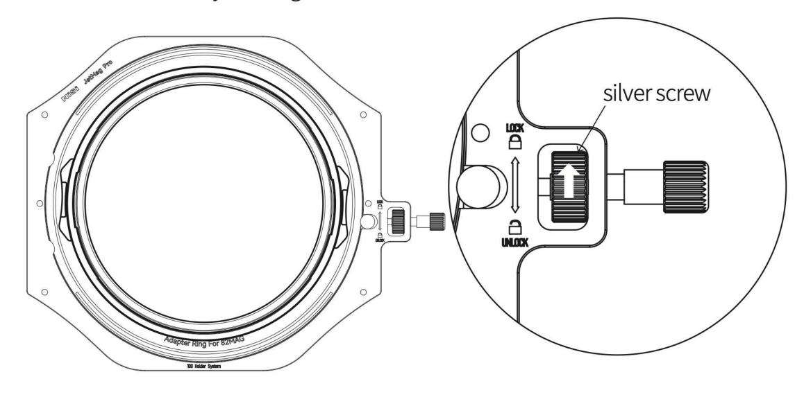
3. Align the side of the 82MAG holder adapter with the white line facing the camera. Align with the section of the holder adapter that does not have white markings (magnetic connection point).
